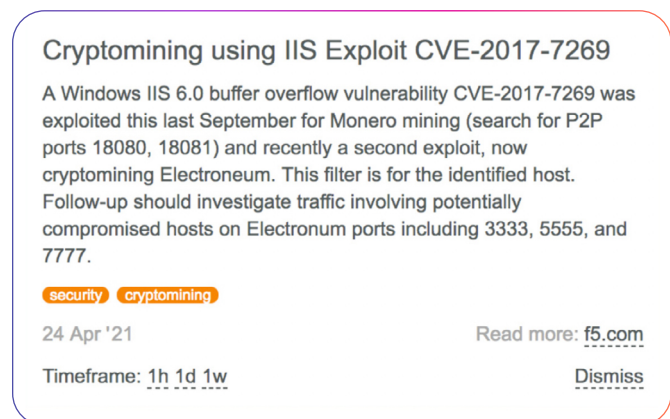
Figure 2. An example of a threat feed. You can read more about it, or explore your environment for signs Electroneum on ports 3333, 5555, or 7777 in the past 1 hour, 1 day, or 1 week.
